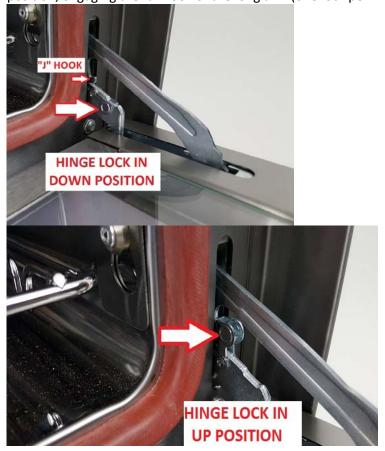
3. Tilt the door up at a 45-60 degree angle (hinge lever arm will be released)
