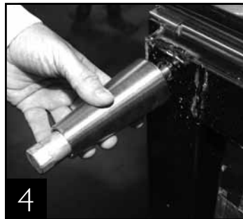
4 Thread leg into cabinet bottom frame rail.
